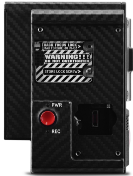
Figure: Do NOT Lock Back Focus When Adjusting Back Focus
